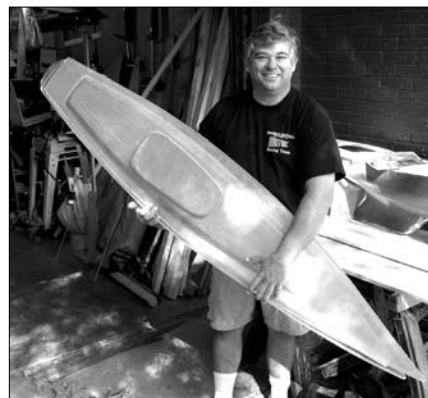
Larry is holding together a fresh-from-the-mold, Ocean Racer-style deck, along with a fresh-from-the-mold S/B hull. Photo by Rich Matt.
